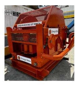
The 32mT SWL hydraulically winch is manually operated. There are no electrical components, the brake and gears are fully enclosed, making the winch suitable to operate in hazardous zone II environment. The winch is fitted with a fail-safe brake, meaning that the brake will always be engaged in case of pressure drop. Typical use for this winch:
