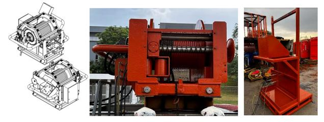
The 20mT SWL hydraulically winch is manually operated. There are no electrical components, the brake and gears are fully enclosed, making the winch suitable to operate in ATEX zone II environment. The winch is fitted with a fail-safe brake, meaning that the brake will always be engaged in case of pressure drop.
